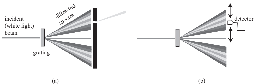
Figure 8.1 Use of a diffraction grating (a) as a monochromator and (b) as a spectrometer.
