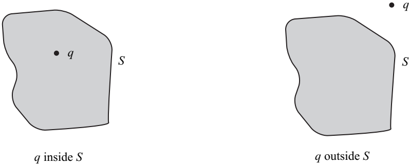
Figure 6.1 A charge inside and outside of the closed surface S .
