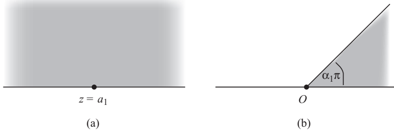
Figure 10.15 Illustrating a mapping from (a) the upper half of the z -plane to (b) a wedge domain in the w -plane with opening angle \alpha_1 \pi .
